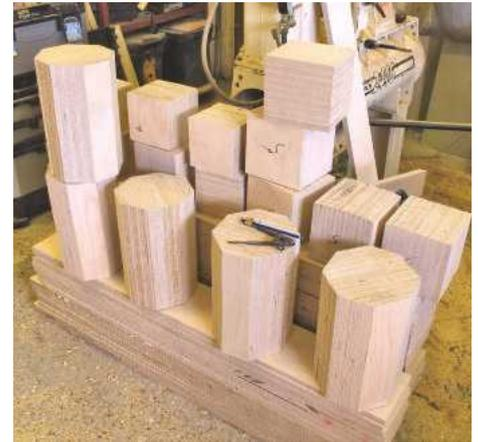
▲ Pic.3 This is about a third of the blanks needed. Les cut them to length on the bandsaw. He found that a narrow kerf blade cut the plywood better
